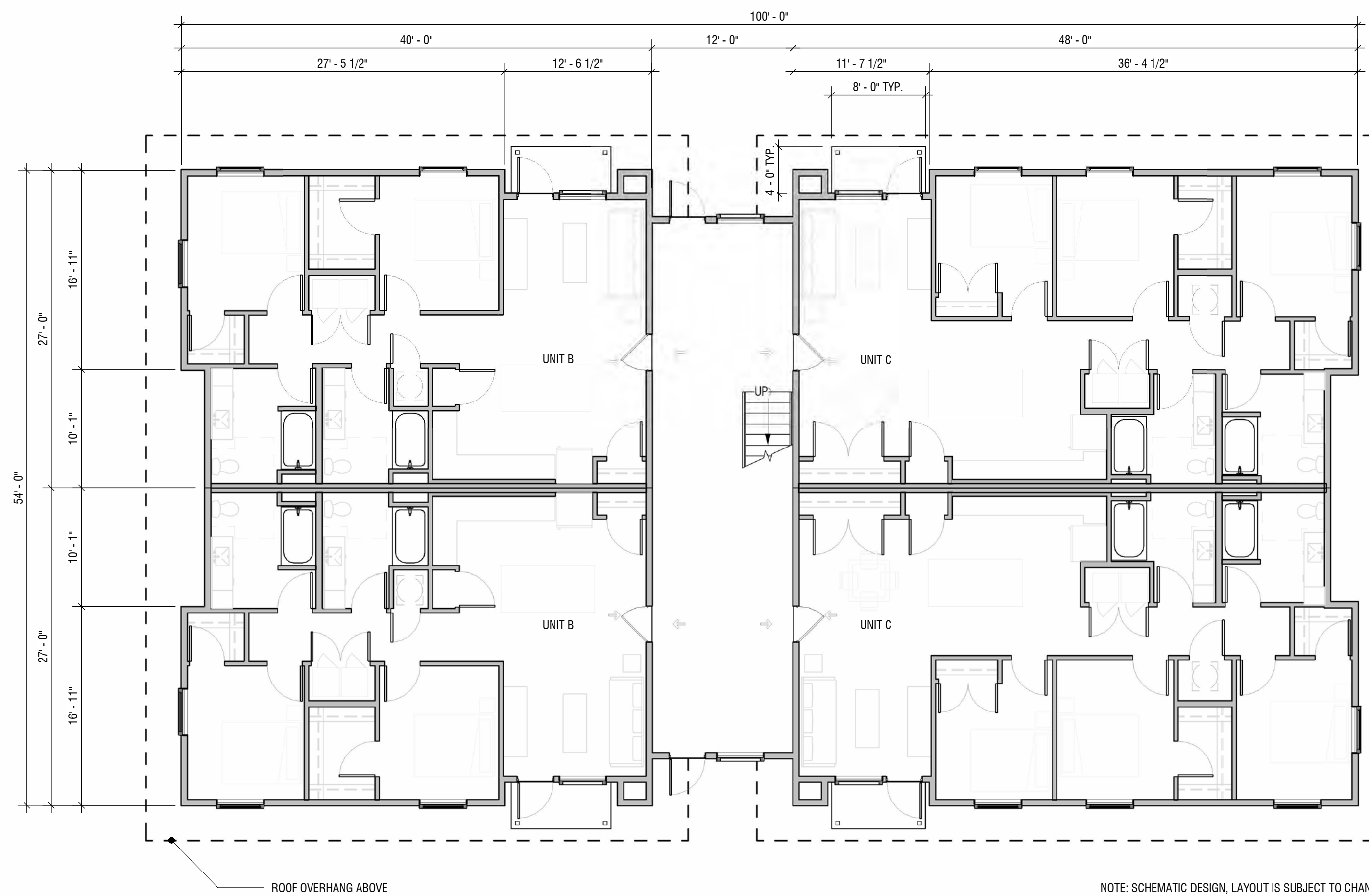
2 BUILDING TYPE B FLOOR PLAN A02 1/8" = 1'-0"
